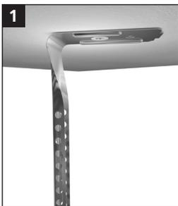
1 Mark the fixing points on the ceiling in accordance with the table "Suspension point dimensioning for ceiling installation". Fix the vernier hanger top part to the ceiling. After fixing the vernier hanger, bend it by 90° into a vertical position.
