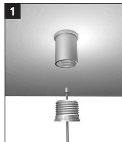
Mark the fixing points on the ceiling in accordance with the table "Suspension point dimensioning for ceiling installation". Fix the ceiling fixing M13 x 1 to the ceiling. Lead the steel wires through the screw cap M13 x 1. Then screw the cap M13 x 1 to the ceiling attachment M13 x 1.
